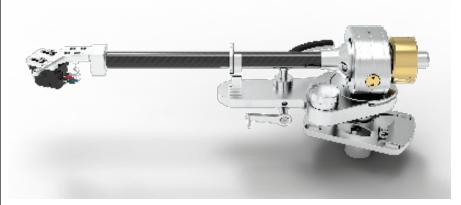
different. The internal wiring on both arms is made from 4N silver, selected for its exceptional flexibility to minimize any effect on the arm's freedom of movement, in both planes. A 5-pin DIN connector at the base of each arm allows you to connect the included Equator Achromatic cable, from Atlas Cables of Scotland. Standard, singleended RCA connectors and balanced XLR connectors are available.
